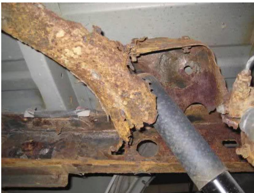
23. The Frames on the Vehicles are materially the same for purposes of this class proceeding and suffer from the same Design Defect. All of the Frames were manufactured by the same corporation (namely, Dana Holding Corporation) pursuant to the same defective manufacturing and design process. Further, the Toyota Sequoia is based on the Toyota Tundra, sharing an identical frame and frame assembly.
