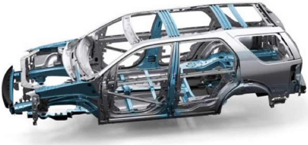
19. The function of vehicle frames includes handling static and dynamic loads with unintended deflection and distortion, preventing undesirable forces and twisting from driving over uneven surfaces, engine torque, vehicle handling and accelerating and decelerating. Frames also are the primary component that guard against sudden impacts and collisions.
