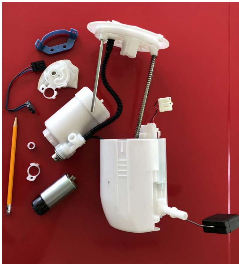
32.5 The fuel pump module's housing protects the fragile internal components that fit together very specifically (like puzzle pieces) within the module and is held together with plastic tabs and clips:
