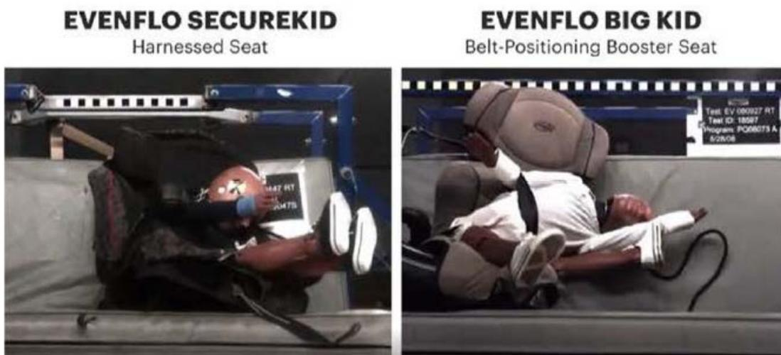
26. As can be seen above, in the test of the SecureKid, the dummy's head and torso remained entirely within the seat's confines. By contrast, in the test of the Big Kid, the seat belt slipped off the dummy's shoulder, and the dummy's head and torso flailed far outside the seat.
