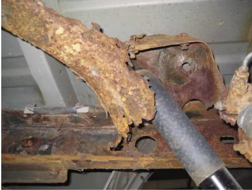
23. The Frames on the Vehicles are materially the same for purposes of this class proceeding and suffer from the same Design Defect. All of the Frames were manufactured and supplied by the same corporation (namely, Dana Holding Corporation) pursuant to the same defective manufacturing and design process. Further, the Toyota Sequoia is based on the Toyota Tundra, sharing an identical frame and frame assembly.
