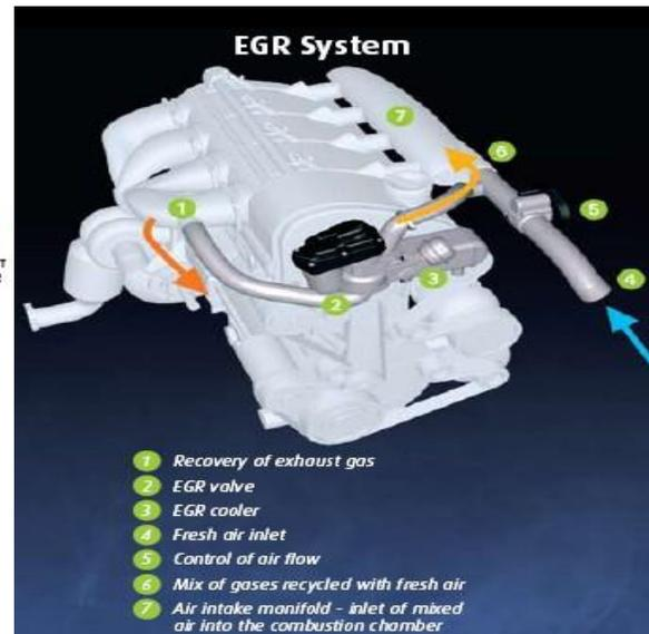
35. Navistar MaxxForce Engines implemented the Advanced EGR system for NOx reduction and a Diesel Oxidation Catalyst (“DOC”) Diesel Particulate Filter (“DPF”) for reduction of particular matter;
