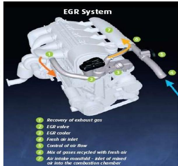
48. Navistar MaxxForce Engines implemented the Advanced EGR system for NO<sub>x</sub> reduction and a Diesel Oxidation Catalyst (“DOC”) Diesel Particulate Filter (“DPF”) for reduction of Particular Matter.
